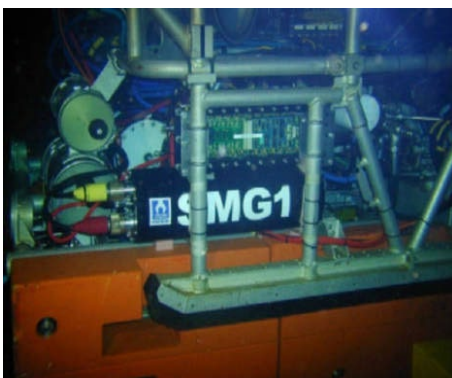
IMES SETS SMG pod mounted on the ROV
